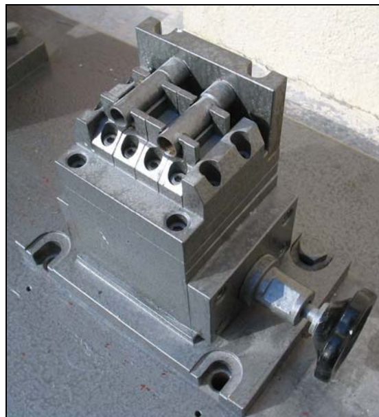
Figure 6. The device with the two centering and fastening mechanisms.
